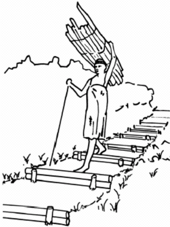
Figure 5. Typical timber pole or bamboo steps
